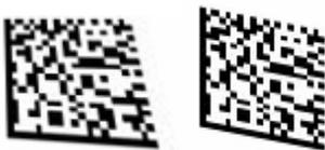
Grid non-uniformity refers to a symbol's cell deviation from the ideal grid of a theoretical perfect symbol. The greatest distance from an actual to a theoretical grid intersection determines the grid non-uniformity grade.
